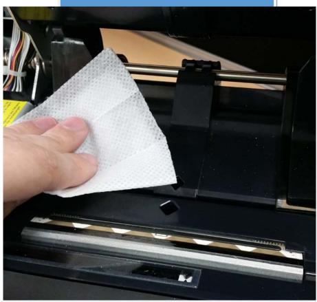
Ensure that all the paper dust and debris is carefully removed using a General Purpose Wipe or General Cleaning Spray and a Lint Free Cloth.
