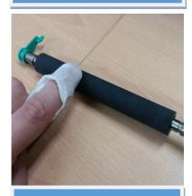
3. Remove the roller from printer and clean using Platen Cleaner Spray and a Lint Free Cloth.
