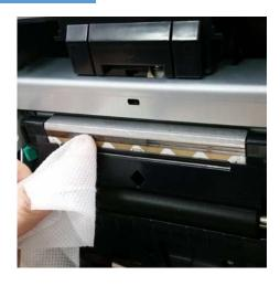
Using a Print Head Cleaning Wipe, ensure that all the paper dust and debris is carefully removed from print heads. Clean using a gentle left to right motion.
