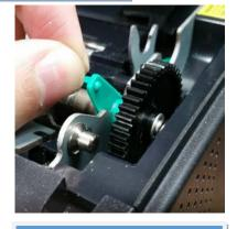
2. Locate and carefully lift the small green levers at both ends of the roller.
