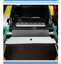
4. Insert the roller back into the printer. Ensure that the green levers are slotted in the metal guide slots.
