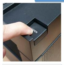
1. Open the printer lid by pressing and releasing the OPEN button.
